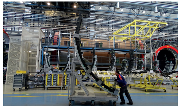
Positioning of aerostructure frames
